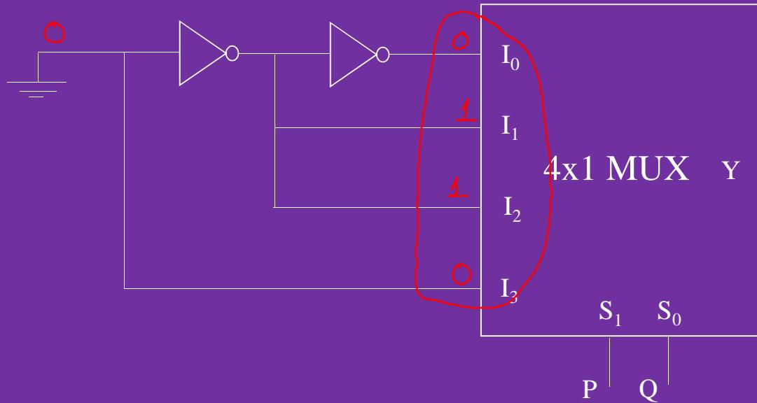
$$\begin{aligned} F &= 0 \cdot \bar{P} \bar{Q} + 1 \cdot P \bar{Q} \\ &\quad + 1 \cdot \bar{P} \cdot Q + 0 \cdot P \cdot Q \\ &= P \bar{Q} + \bar{P} Q = P \oplus Q \end{aligned}$$
