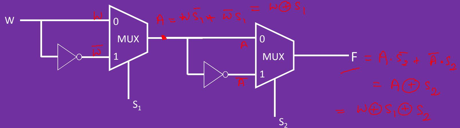
Which of the following Boolean functions is realized by circuit ?
